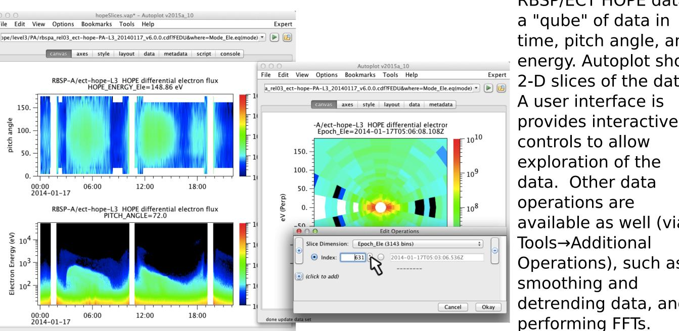
time, pitch angle, and energy. Autoplot shows 2-D slices of the data. A user interface is provides interactive controls to allow exploration of the data. Other data operations are available as well (via Tools→Additional Operations), such as smoothing and detrending data, and performing FFTs.
