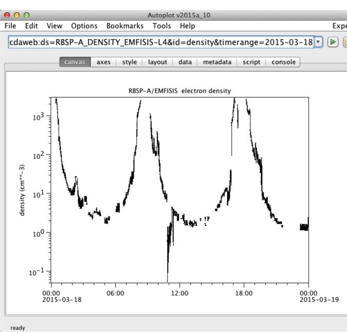
The CDF file for the time requested is downloaded, and parameter displayed. Additional data will be loaded as the time axis is adjusted.
