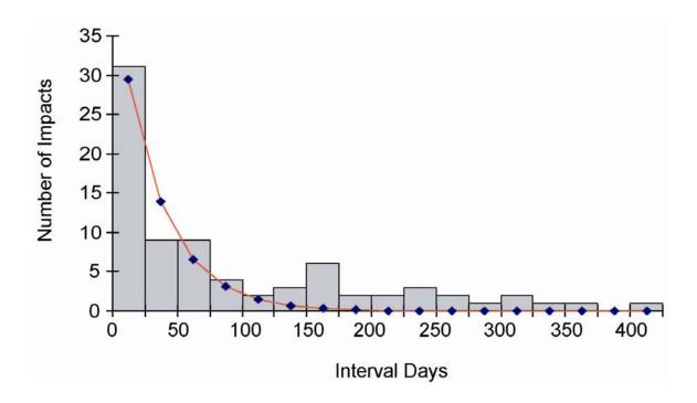
Figure 12. The best-fit Poisson distribution ( $N_m = N_0 e^{-\gamma \Delta t}$ ) of intervals between impacts.  $N_0 = 36.98$  and  $\gamma = 0.0159~s^{-1}$  for both Voyager 1 and Voyager 2. The grey columns represent observed data and the line with spots shows Poisson fit.
