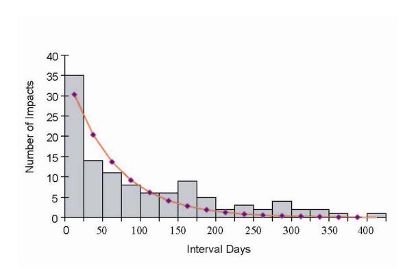
Figure 13. The best-fit Poisson distribution ( $N_m = N_0 e^{-\gamma \Delta t}$ ) of intervals between impacts.  $N_0 = 17.78$  and  $\gamma = 0.0107$  s<sup>-1</sup> for both Voyager 1 and Voyager 2 after 1986. The grey columns represent observed data and the line with spots shows Poisson fit.
