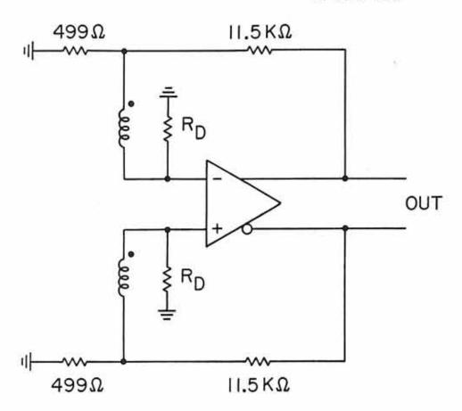
Figure 14. A block diagram of the Polar and Wind search coil preamplifier when a differential signal is applied at the inputs.
