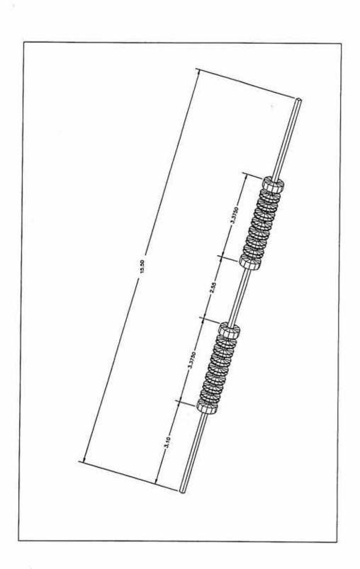
Figure 8. A sketch of the Polar and Wind search coil bobbins. Dimensions are given in inches.
