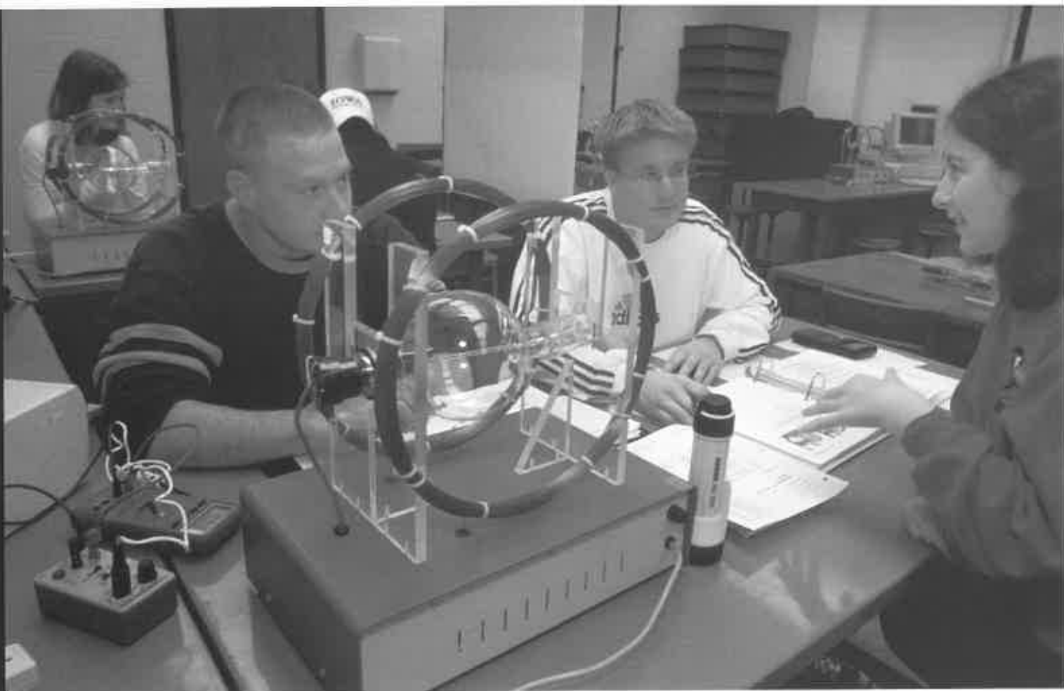
Most teaching assistants supervise an undergraduate lab. Here, a physics TA explains the e/m experiment to two undergraduates. These teaching labs are all equipped with modern instrumentation.
