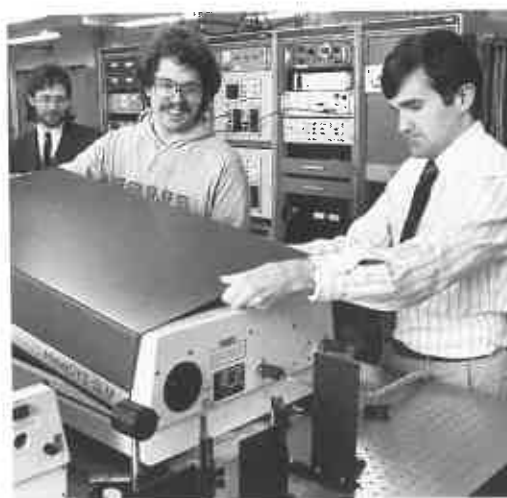
Professor John Goree (right) and associates work on laser used for measurements of ion distribution functions in plasmas
