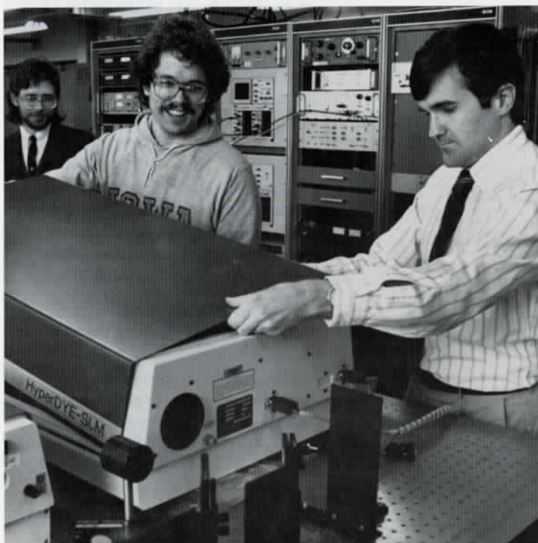
Professor John Goree (right) and associates work on a laser used for measurements of ion distribution functions in plasmas.
