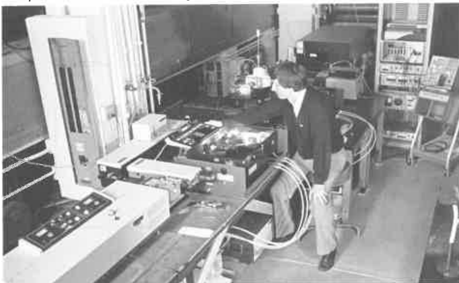
Professor William Stwalley studies laser-induced plasmas and metal vapors with a microprocessor-controlled Nd:YAG/Dye laser
