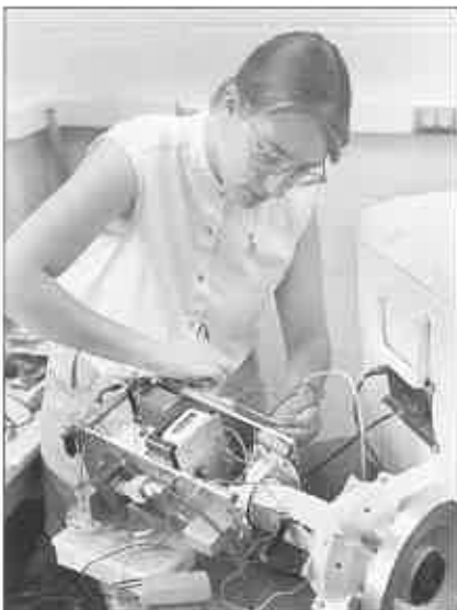
Student Brita Neller installs a switch on a 6 cm radiotelescope receiver
